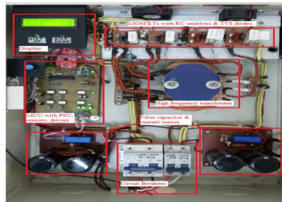
Figure 9. Photograph of the developed isolated bi-directional DC-DC converter.
